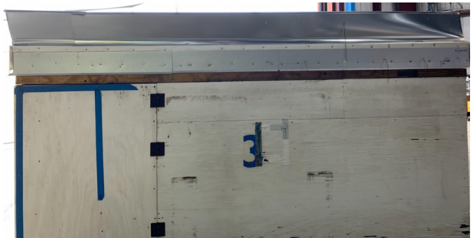
FIGURE 10: Photo of failure mode of Configuration #1.
