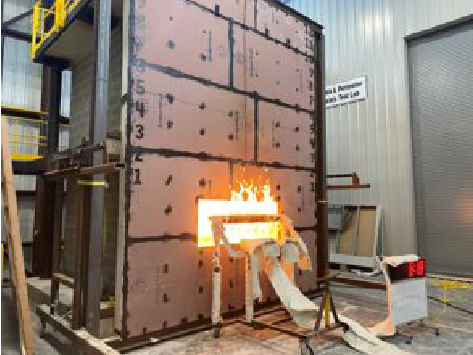
FIGURE 8. NFPA 285 wall assembly while burning from both the exterior and interior.
