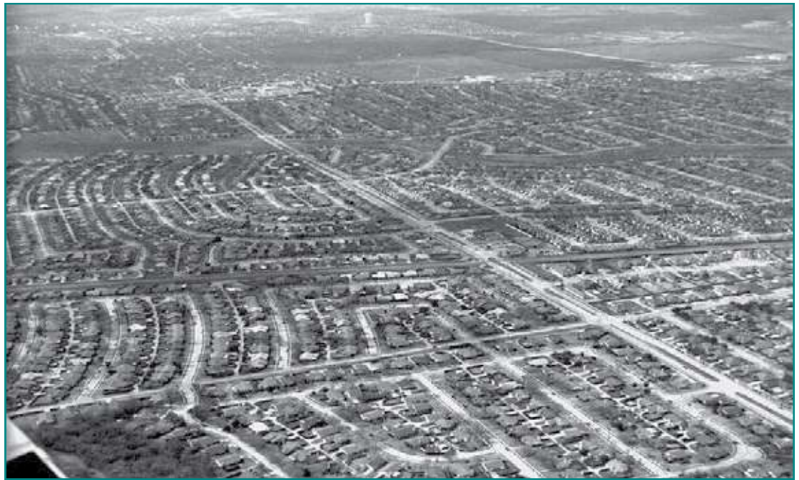
Figure 1 – Example of Exposure B: suburban residential area with mostly single-family dwellings and low-rise structures less than 30 ft. high. (Photo courtesy of American Society of Civil Engineers.)
