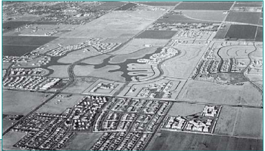
Figure 2 – Example of Exposure C: open grassland with scattered obstructions having heights less than 30 ft. (Photo courtesy of American Society of Civil Engineers.)
