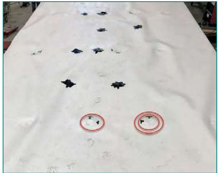
Figure 12 – The two failure locations for Test #4. The double red circle is where the fastener plate pulled over the fastener; the single red circle is the location of the membrane separation at the reinforcement layer.
