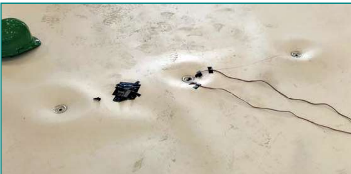
Figure 9 – Circular permanent upward membrane deformation due to two-directional loading in Test #2.
