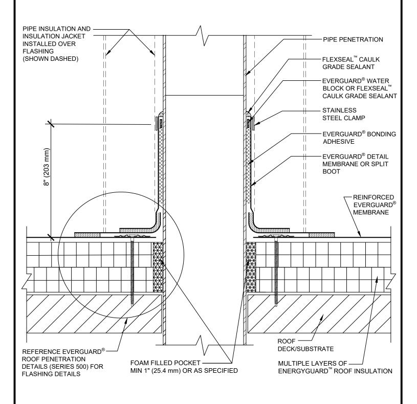
INSULATED PIPE PENETRATION DETAIL WITH FLASHING
