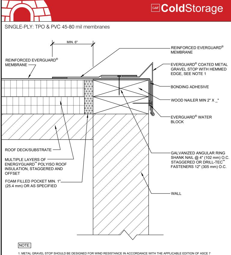
1. METAL GRAVEL STOP SHOULD BE DESIGNED FOR WIND RESISTANCE IN ACCORDANCE WITH THE APPLICABLE EDITION OF ASCE 7 AND TESTED FOR CAPACITY IN ACCORDANCE WITH THE TEST METHODS IN THE APPLICABLE EDITION OF ANSI/SPRI ES-1.
