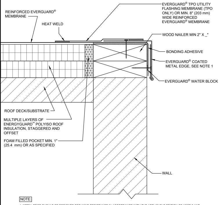
1. METAL EDGE SHOULD BE DESIGNED FOR WIND RESISTANCE IN ACCORDANCE WITH THE APPLICABLE EDITION OF ASCE 7 AND TESTED FOR CAPACITY IN ACCORDANCE WITH THE TEST METHODS IN THE APPLICABLE EDITION OF ANSI/SPRI ES-1.
